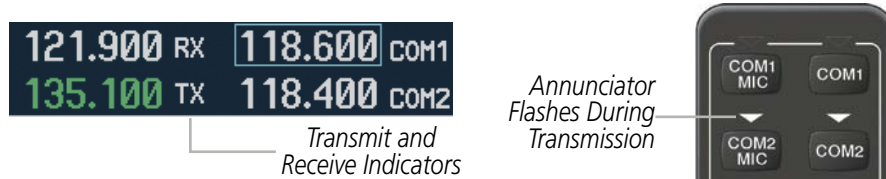
Figure 4-4 COM Radio Transmit and Receive Indications
